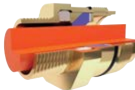
Figure 2 - When a larger diameter cable is installed the inner compensator operates to a greater extent.
